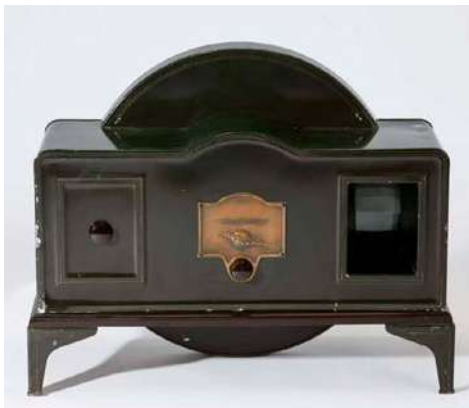
Baird 'Tin Box' television with its tiny screen on the right. About one thousand were sold to wealthy customers who would be able to watch Baird/BBC broadcasts between 1929 and 1935. Source: Public Domain.
